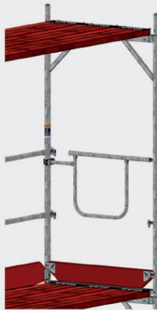
Figure 33: Installed front guardrail: open tube end mounted on a gravity lock
